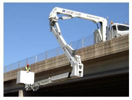
controlled basket that can be used for access beneath a bridge from the roadway. The District would purchase a snooper truck which operates within a single lane closure and that has a reach to span over the sidewalk and reach down to the net. Several manufactures make such a unit. One example is the Aspen A-62, manufactured by Aspen Aerials, Inc.
