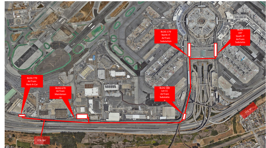
Highlight of 12BAAT-1 12kV path and 12AT-1, and 12AT-2.
