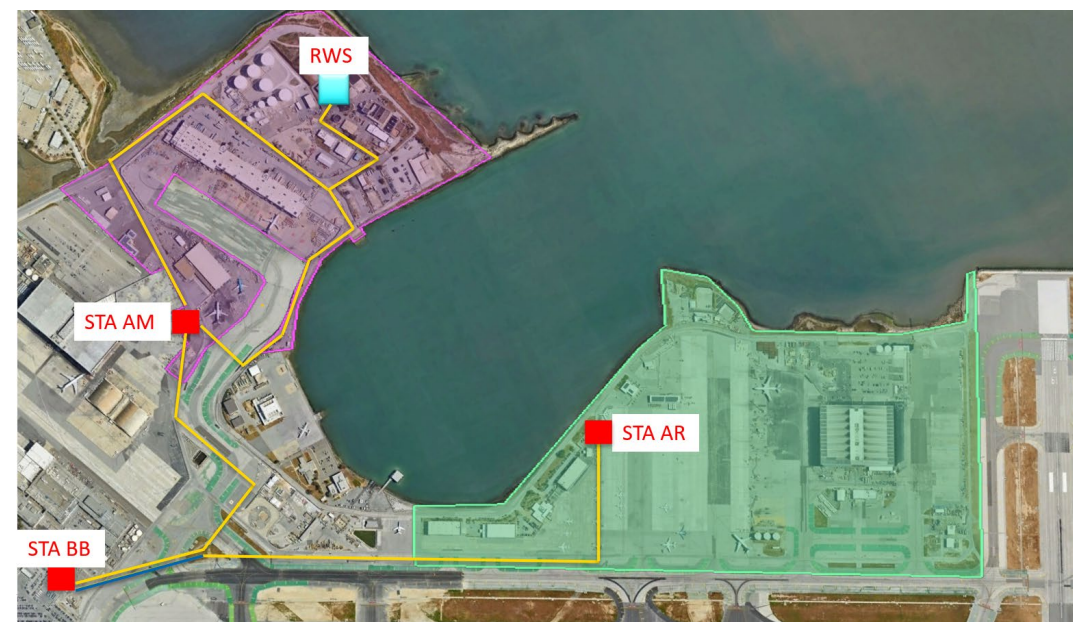
Underground 12kV duct bank routes between Stations and a Facility
