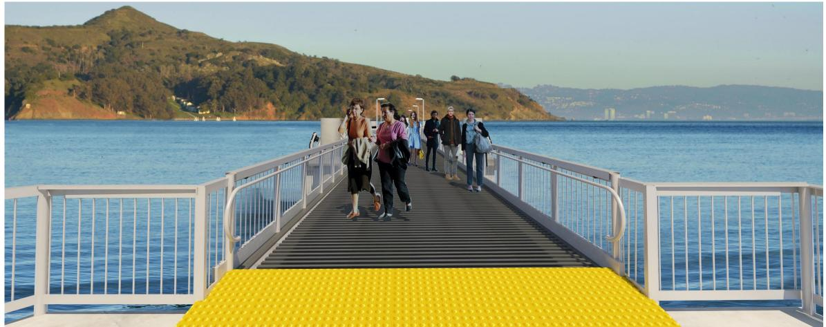
Changes made in 2017: Reduced width and length of float, reduced width of gangway, reduced float light pole height by 1 foot, added bird safety treatment to gate doors
