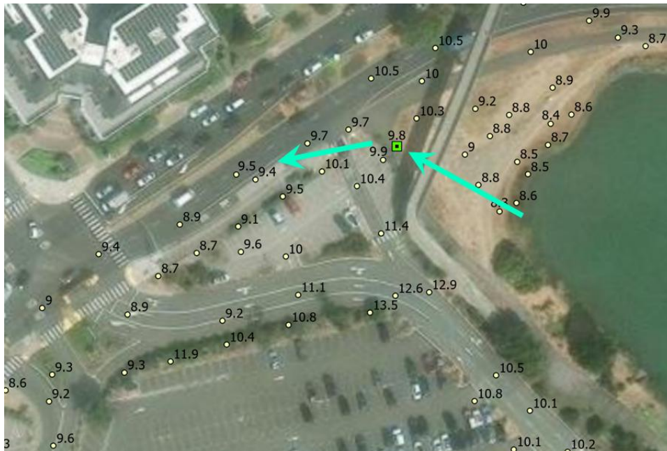
Figure 32. Location and elevation of the floodwater breaching point (■) in Sir Francis Drake Boulevard area at the eastern end of Sir Francis Drake Boulevard by the pedestrian bridge and elevations in the vicinity
