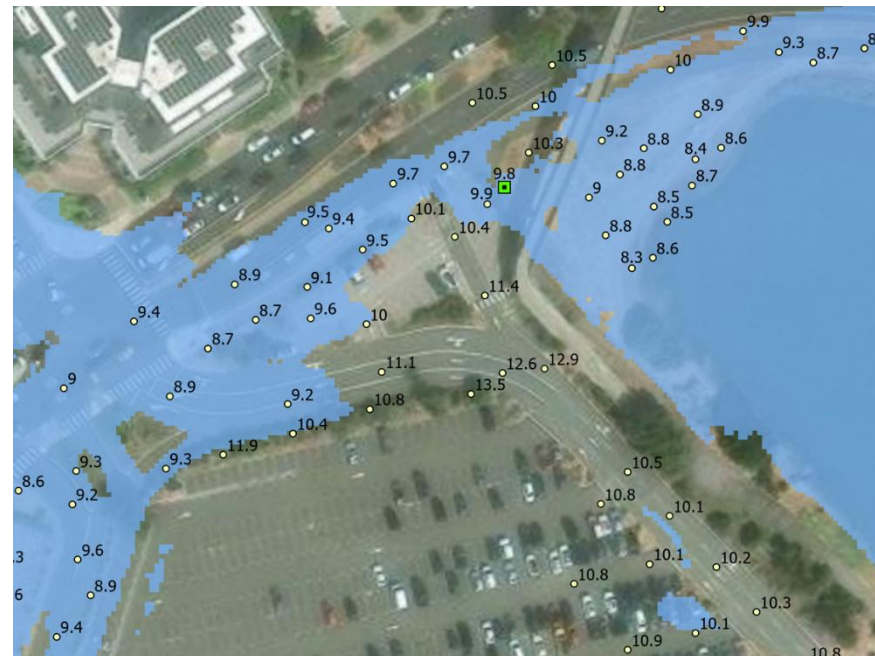
Figure 59. Potential extent of flooding in the Sir Francis Drake Boulevard area assuming infinite duration of the projected 10.2 feet NAVD88 TWL by 2080 (intermediate risk aversion) overtopping the 9.8 feet NAVD88 breaching point and adjacent low-lying areas
