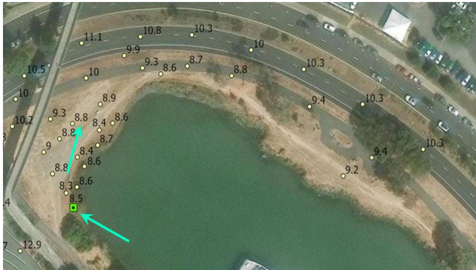
Figure 31. Location and elevation of the floodwater breaching point (■) in the Undeveloped area at the northwest corner of the Larkspur Ferry Terminal basin and elevations in the vicinity
