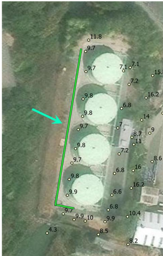
Figure 34. Location and elevation of the floodwater breaching section (red line) in the Fuel Tanks area on the top of the west side of the levee and elevations in the vicinity
