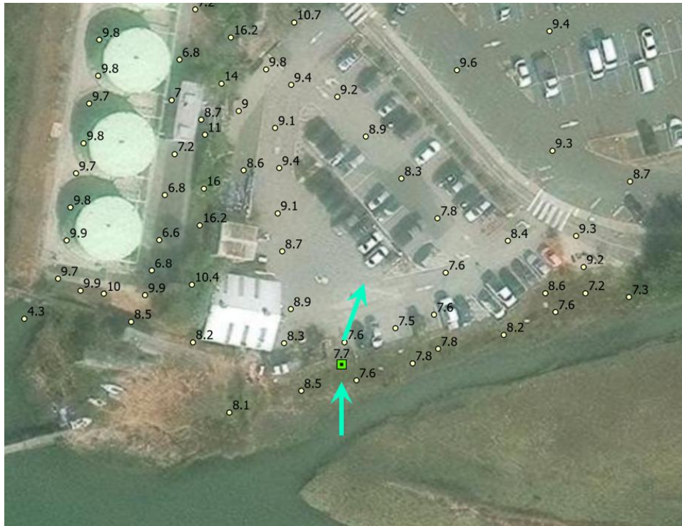
Figure 35. Location and elevation of the floodwater breaching point (7.7) in the Butler Building area at the western landward edge of the marsh close to the Butler Building and elevations in the vicinity.
