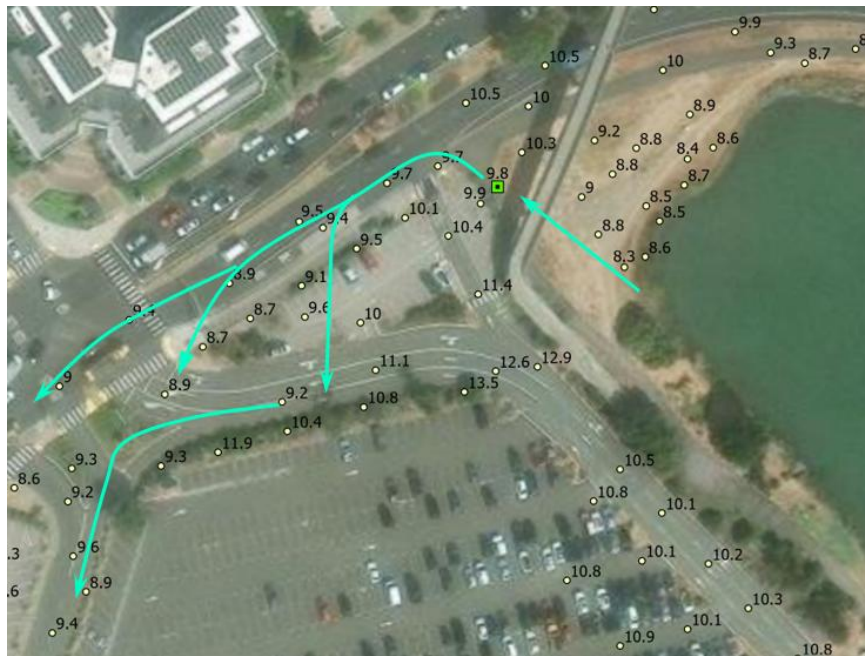
Figure 58. Schematic of potential floodwater pathways in the Sir Francis Drake Boulevard area for the projected 10.2 feet NAVD88 TWL by 2080 (intermediate risk aversion) overtopping the 9.8 feet NAVD88 breaching point
