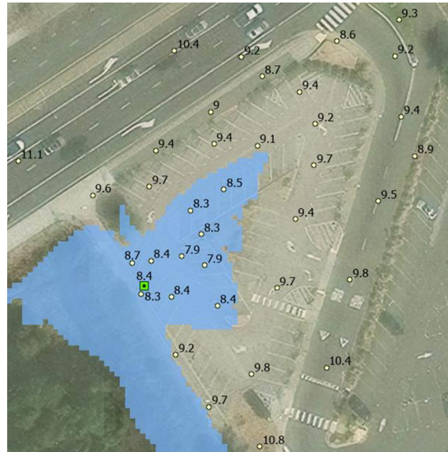
Figure 44. Potential extent of flooding in the Creek area assuming infinite duration of the projected 8.9 feet NAVD88 TWL by 2030 (intermediate risk aversion) overtopping the 8.4 feet NAVD88 breaching point and adjacent low-lying areas
