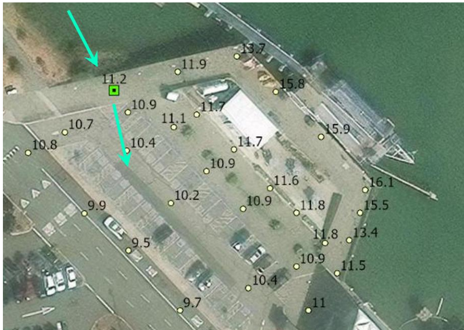
Figure 30. Location and elevation of the floodwater breaching point (■) in the Larkspur Ferry Terminal Buildings area at the northern end of Berth 3 and elevations in the vicinity
