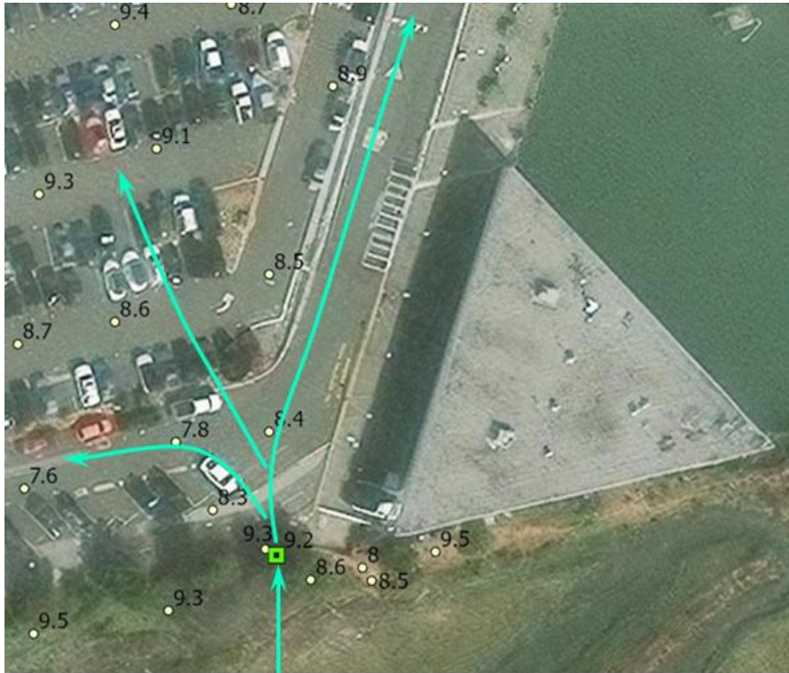
Figure 49. Schematic of potential floodwater pathways in the Marsh area for the projected 9.3 feet NAVD88 TWL by 2050 (intermediate risk aversion) overtopping the 9.2 feet NAVD88 breaching point
