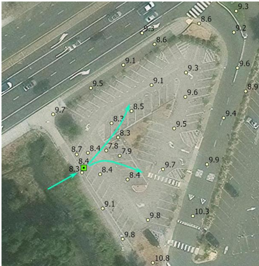
Figure 43. Schematic of potential floodwater pathways in the Creek area for the projected 8.9 feet NAVD88 TWL by 2030 (intermediate risk aversion) overtopping the 8.4 feet NAVD88 breaching point
