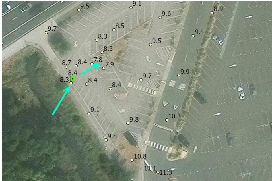
Figure 33. Location and elevation of the floodwater breaching point (■) in the Creek area near the northern end of the Creek and elevations in the vicinity
