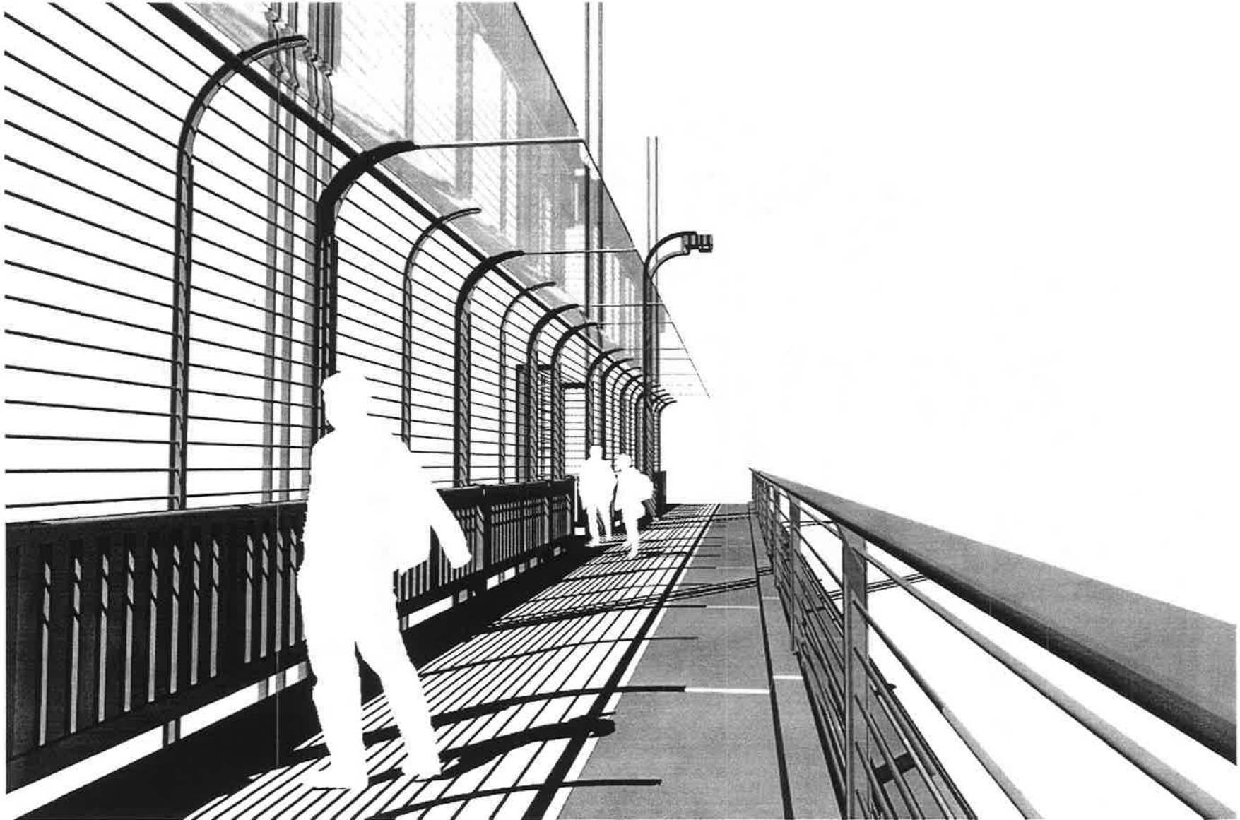
FIGURE 1.3b - EXAMPLE OF CONCEPT 1 (EXAMPLE SHOWN WITH HEIGHT OF 12'-0" TRANSPARENT WINGLET OF 64", HORIZONTAL MEMBERS SPACED AT 6", SOLID RATIO OF 9%) VIEW FROM SIDEWALK
