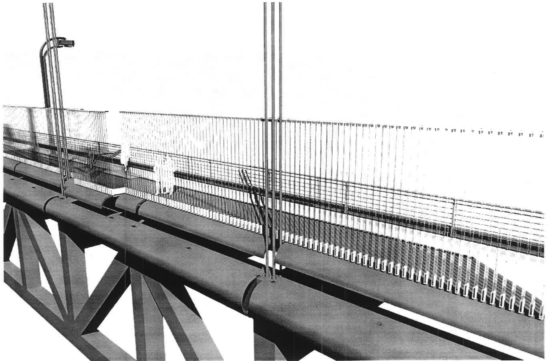
FIGURE 2.6b - EXAMPLE OF CONCEPT 2 (EXAMPLE SHOWN WITH HEIGHT OF 12'-0", NO WINGLET; WIND FAIRINGS ON TRUSS AND SIDEWALK, VERTICAL GLASS PICKETS SPACED AT 7", SOLID RATIO OF 23%) VIEW FROM OUTBOARD
