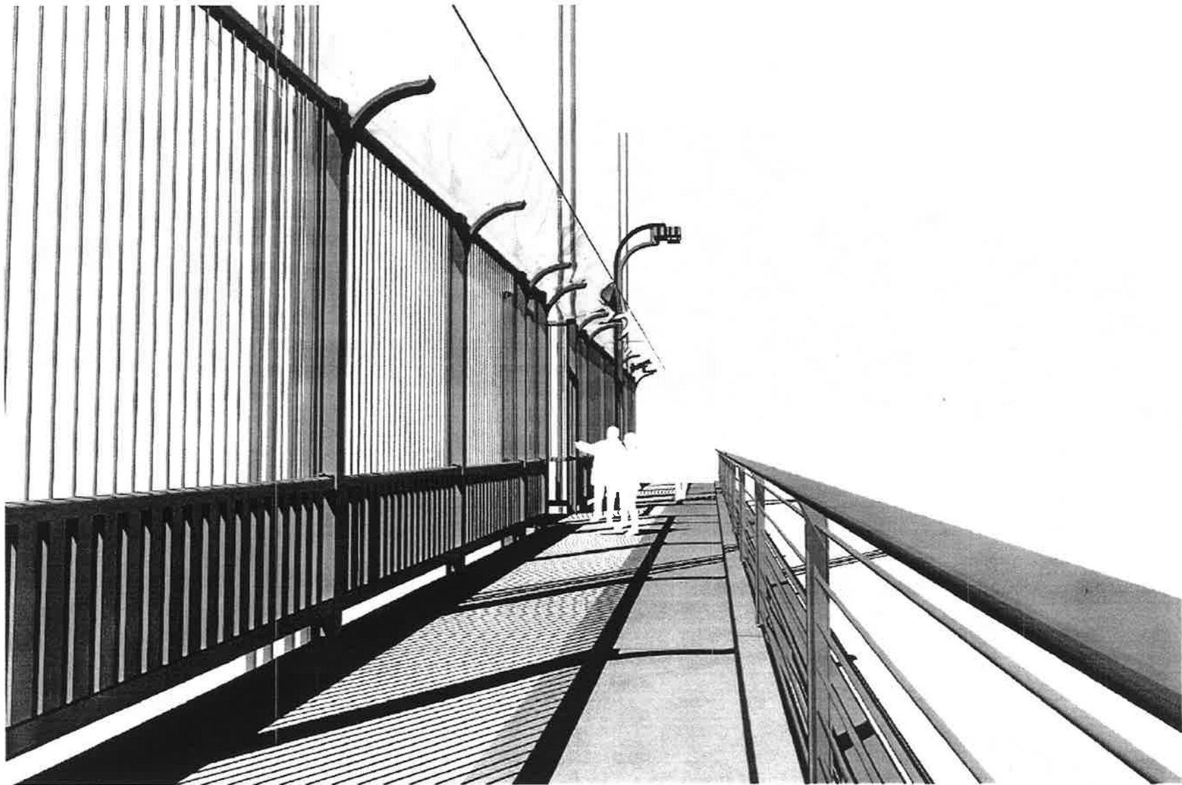
FIGURE 1.2b - EXAMPLE OF CONCEPT 1 (EXAMPLE SHOWN WITH HEIGHT OF 14'-0" TRANSPARENT WINGLET OF 64", VERTICAL MEMBERS SPACED AT 6", SOLID RATIO OF 12%) VIEW FROM SIDEWALK
