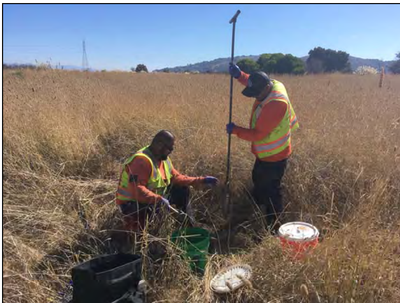
Photograph 5: View of field team members advancing a soil boring using a hand auger in sample grid cell D8, looking southeast. October, 2018.
