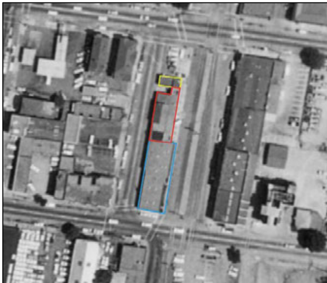
Figure 6. 1965 aerial image. The red border represents the remaining original passenger waiting room and enclosed passenger arcade along its east side; the blue border represents the south office addition (1940s); the yellow border represents the north office addition (1950s). Source: University of California, Santa Barbara Library (Flight CAS_65_130, Frame 39-185), edited by ICF.
